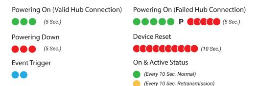
**NOTE:** If the Sensor is out of range or the Hub unit was not turned on, the status LED on the Sensor will start rapidly blinking red after power up. Make sure the Hub unit was turned ON first or try relocating the Sensor/Hub combination so they are closer to each other. Power cycle or reset Sensor to retry Hub unit connectivity validation. (For further troubleshooting refer to hardware user manual)
