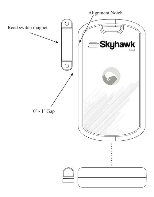
**Reed Switch Magnet** - This device is to be used as an accessory in conjunction with the reed switch sensor built into the Kiwi. The reed switch can be used as an alternate event trigger when separated from the unit.
