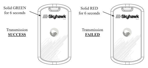
**Step 4**: After the trigger the unit will return to power savings mode. It will not be ready for the next trigger until after the specified times set in the **Alert Interval Options** in the app.
