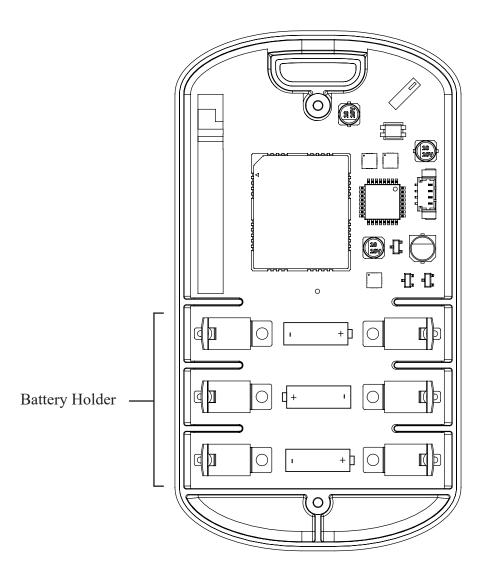
*Battery Holder* - The battery holder accommodates 3 x AAA batteries. It is required that 1.5 volt lithium batteries, like an Energizer Advanced Lithium or Ultimate Lithium, are used for expected life.
