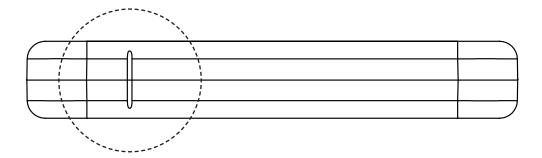
**Step 3:** Peel the backing off the magnet mount and affix to the side of case as shown. The mount should be centered on the notch.
