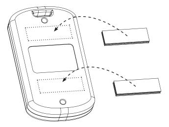
**Step 4:** Make sure the area where the Kiwi will be attached has a clean surface for proper bonding of the strips. Do not separate the strips from the back of the unit at this time!
