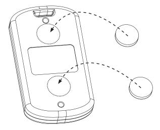
**Step 4:** The Kiwi is ready to be mounted. Make sure the area where the Kiwi will be attached is ferrous iron or steel.
