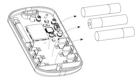
Step 4: Insert new batteries taking note of the direction symbols.
