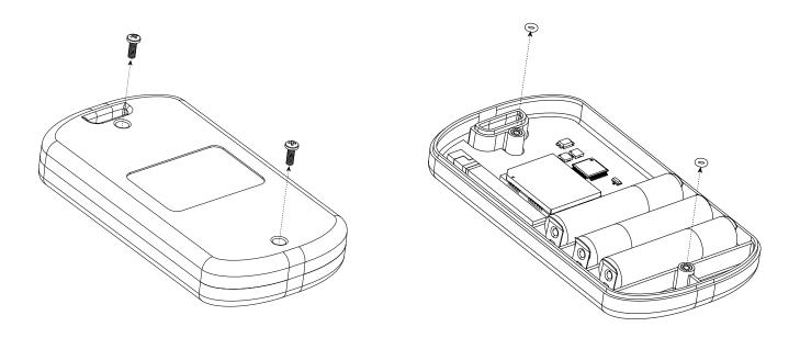
**Step 2**: Remove the rear cover. There may be a gasket holding the unit together so it might take a bit of force to separate the rear cover from the front. There will also be two small O-rings between the two covers at the screw hole locations. Be sure not to misplace these as they provide the water-tight seal for the unit.
